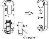
2. Attach the camera to the mounting plate using the lock screw (4x9mm) and L-wrench included with the camera.
